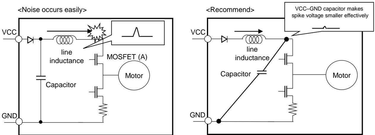
At motor driving, Vcc current flows to MOSFET.
