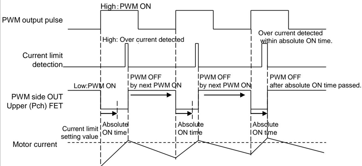
Normal mode(Motor speed > FG frequency 6.67Hz) : Current limit setting voltage = 150mV (Vcs1)
